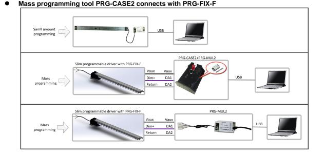
Note: Only the slim DALI driver need AC power when programming in the top diagram(Small amount programming).
