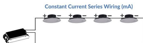
Figure 1: Example of a series wiring using a constant current driver.
